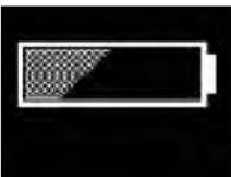
The display showing a half empty battery indicates that it is time to charge the battery.
