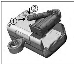
4. Install 6 x AAA size batteries. Ensure correct polarity is observed.
