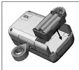
5. Reinstall the battery case as shown.
